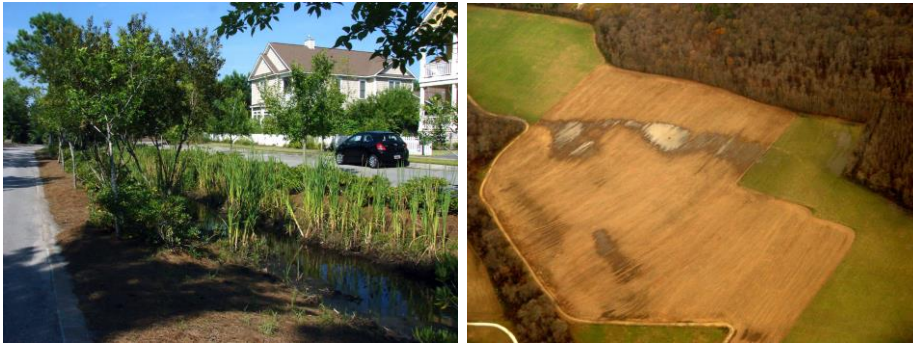
Figures 10a and 10b: The location of this street at Demarest Landing follows what had originally been an ugly ditch. Springtime aerial photos can reveal opportunities hidden from the eye at ground level, particularly during drier parts of the year. Instead of engineering these darker (moister) areas for houselots and streets, they could become the greenway system around which the development is designed. The initial conceptual design stage is precisely when a landscape architect could best contribute to the charrette team.
